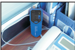
Connect launcher and telephone wire port to be traced in right way
